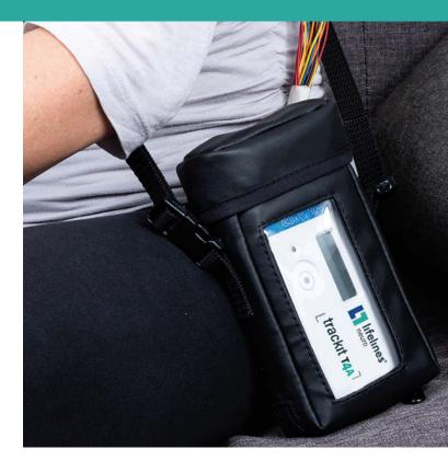
Trackit T4A is a high performance ambulatory EEG recorder for use with Lifelines Neuro's ambulatory systems. It is a low power, battery-operated recorder, with 28 monopolar and 4 user configurable channels, delivering the highest quality EEG for up to 72 hours continuously using Trackit and Trackit Plus software. Data can be read anywhere, anytime using dedicated cloud software.
