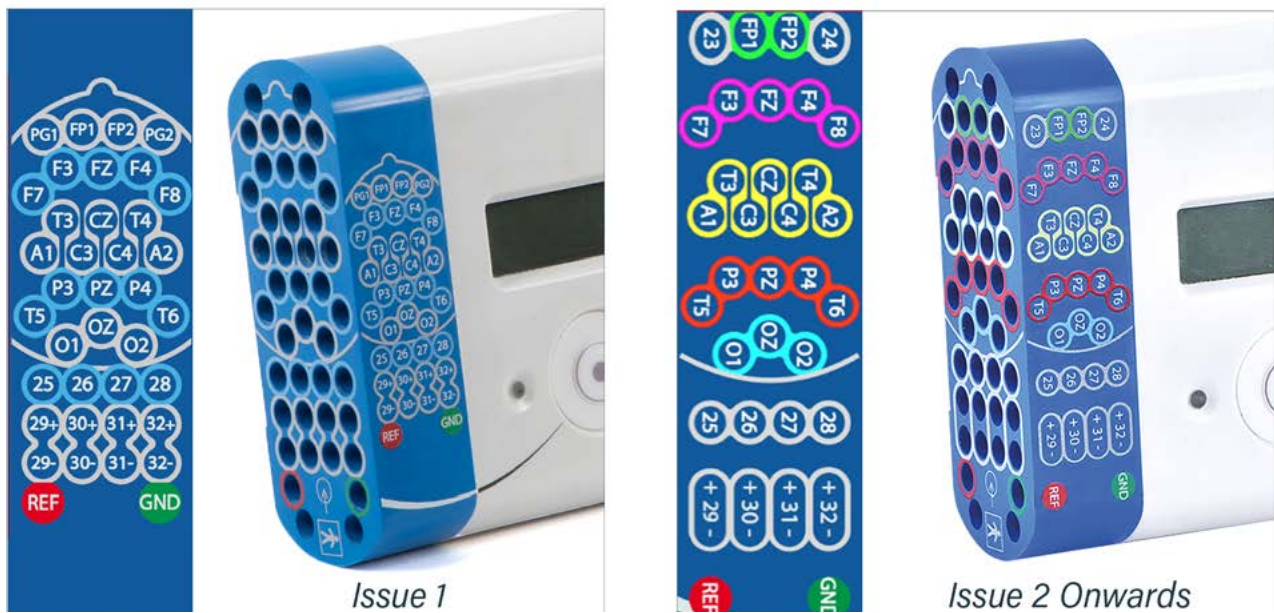
Figure 5: Connecting the Trackit T4A Amplifier (PCU/front face)
