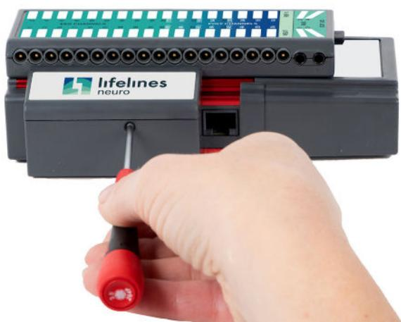
Figure 12: Clickon PCU Retaining screw location
