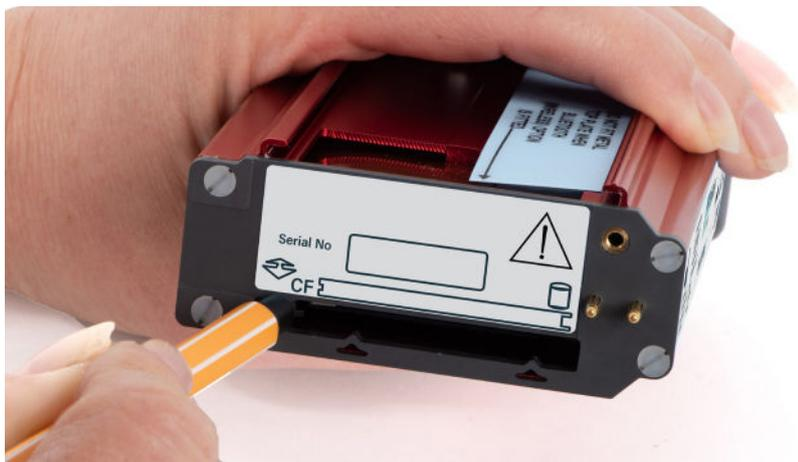
Figure 11: Removing the flash card
