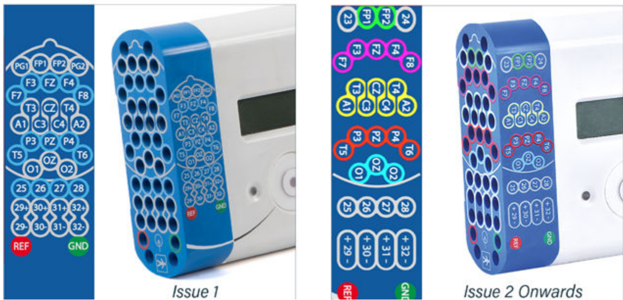
Figure 5: Connecting the Trackit T4A Amplifier (PCU/front face)
