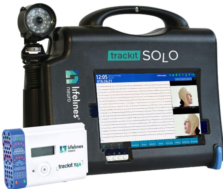
The Trackit T4A is the amplifier of choice for use with the Trackit Solo.
