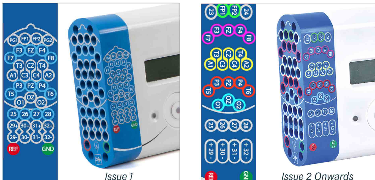
Figure 5: Connecting the Trackit T4A Amplifier (PCU/front face)
